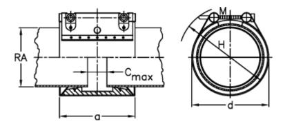
a = 98.0 C max with insertion band = 25 d = 95 H = 115
